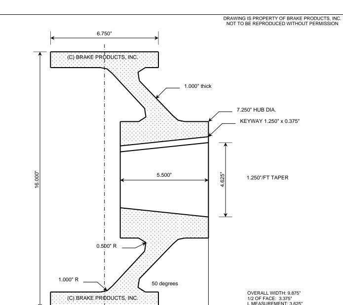
1/2 OF FACE: 3.375" L MEASUREMENT: 3.625" WEB-TO-HUB EXTENSION R: 2.146" FACE-TO-HUB EXTENSION L: 4.375" FACE-TO-HUB EXTENSION R: 3.125" APPROXIMATE WEIGHT (LBS.): 95 SMALL BORE DIAMETER: 4.052"
